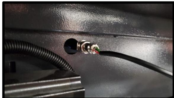
**When you are done using the BossMod, unplug the 4-pin connector for the rotary device and plug back in the original 4-pin connector for the Y-Axis Motor.**
