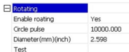
**NOTE:** To go back to the worktable, press the **Read button** > **Change Enable rotating to "No"** > press the **Write button**. Make sure the machine is on and connected to the PC via USB Cable.
