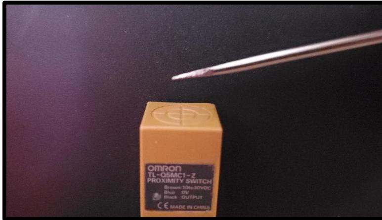
A red LED light should turn on from the front side of the limit switch (where the label is located). This will tell you that the switch is being activated. This will stop the rotary to stop moving for a quick second and try to slowing move again. Touch the limit switch again to properly DATUM (home) the Y-Axis. The rotary is now correctly adjusted with the corresponding coordinates of your worktable and now should be ready to be used.
